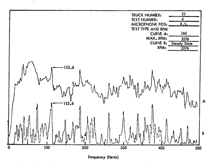
Figure C54. Truck Exterior Noise Spectra (Narrow Band Analysis 1–1/4 Hertz) Measured at 50 Feet. The Spectra Are Used For Determining Engine RPM.
