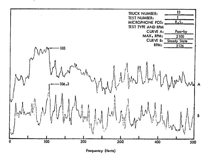
Figure C46 . Truck Exterior Noise Spectra (Narrow Band Analysis 1-1/4 Hertz) Measured at 50 Feet. The Spectra Are Used For Determining Engine RPM.
