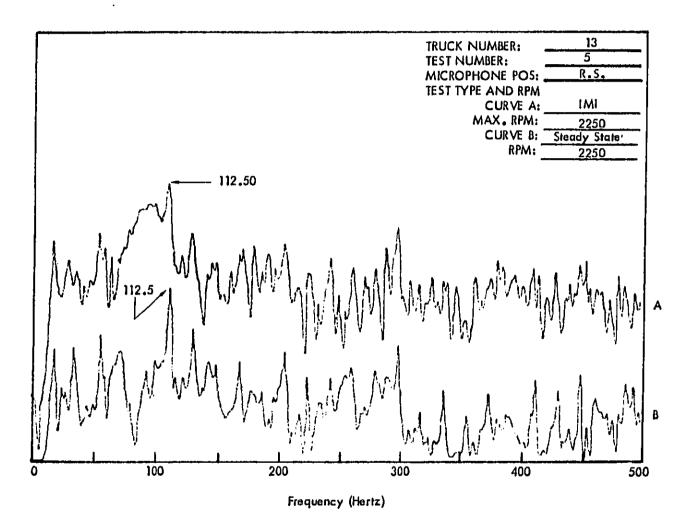
Figure C48. Truck Exterior Noise Spectra (Narrow Band Analysis 1-1/4 Hertz) Measured at 50 Feet. The Spectra Are Used For Determining Engine RPM.
