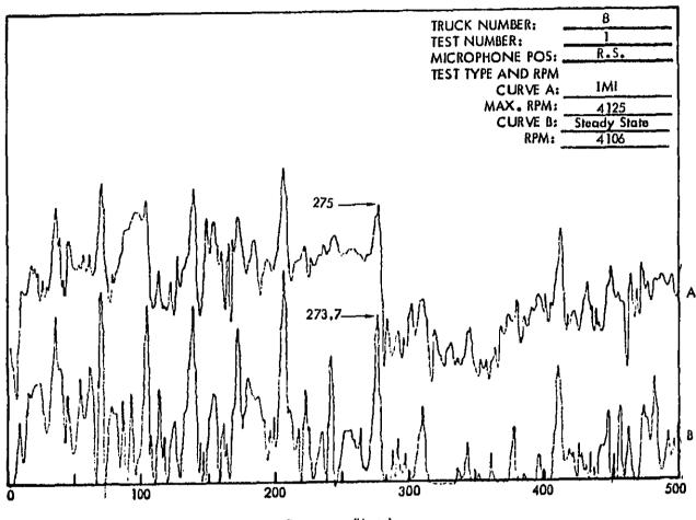
Figure C25. Truck Exterior Noise Spectra (Narrow Band Analysis 1–1/4 Hertz) Measured at 50 Feet. The Spectra Are Used For Determining Engine RPM.
