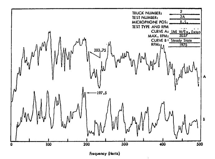
Figure C5. Truck Exterior Noise Spectra (Narrow Band Analysis 1–1/4 Hertz) Measured at 50 Feet. The Spectra Are Used For Determining Engine RPM.
