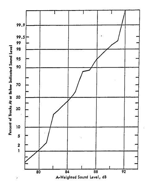
Figure 20. Cumulative Distribution of New Diesel Truck Noise Levels (Reference 10)
