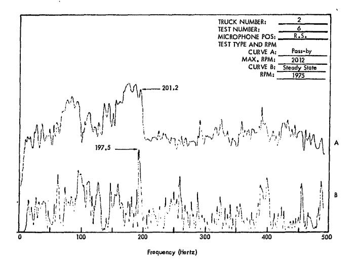
Figure C8 . Truck Exterior Noise Spectra (Narrow Band Analysis 1–1/4 Hertz) Measured at 50 Feet. The Spectra Are Used For Determining Engine RPM.
