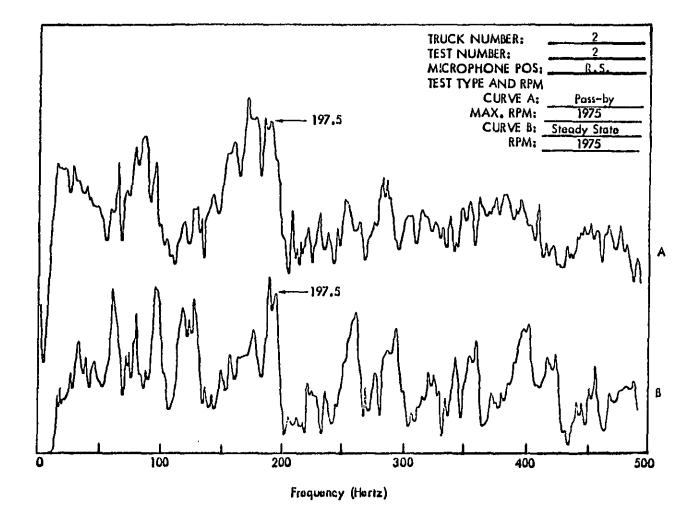
Figure C6 . Truck Exterior Noise Spectra (Narrow Band Analysis 1-1/4 Hertz) Measured at 50 Feet. The Spectra Are Used For Determining Engine RPM.
