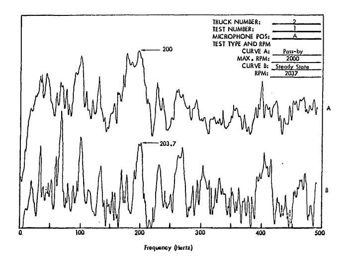
Figure C3 . Truck Exterior Noise Spectra (Narrow Band Analysis 1–1/4 Hertz) Measured at 50 Feet. The Spectra Are Used For Determining Engine RPM.
