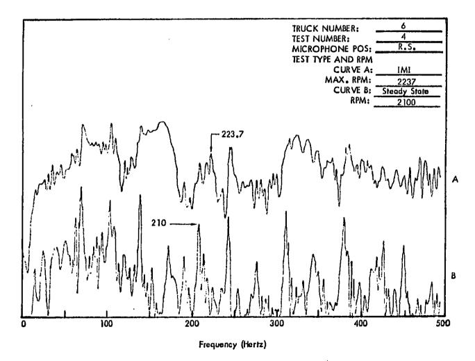
Figure C16 . Truck Exterior Noise Spectra (Narrow Band Analysis 1-1/4 Hertz) Measured at 50 Feet. The Spectra Are Used for Determining Engine RPM.
