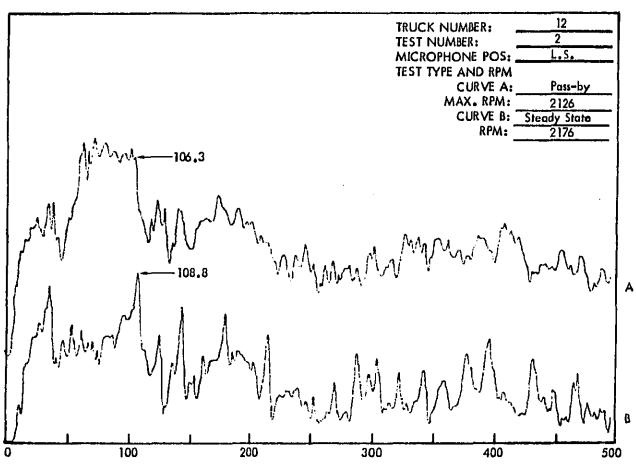
Figure C40. Truck Exterior Noise Spectra (Narrow Band Analysis 1–1/4 Hertz) Measured at 50 Feet. The Spectra Are Used For Determining Engine RPM.
