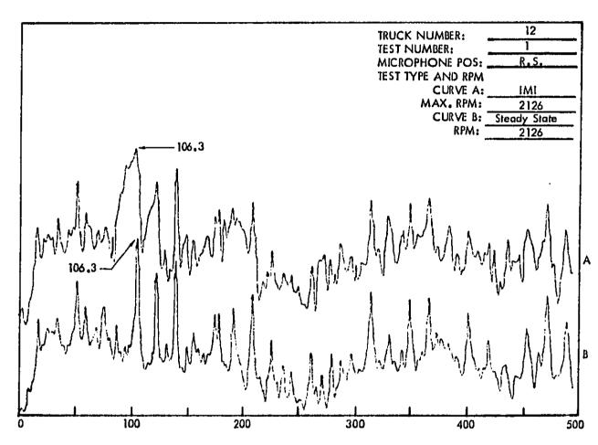
Figure C37. Truck Exterior Noise Spectra (Narrow Band Analysis 1–1/4 Hertz) Measured at 50 Feet. The Spectra Are Used For Determining Engine RPM.
