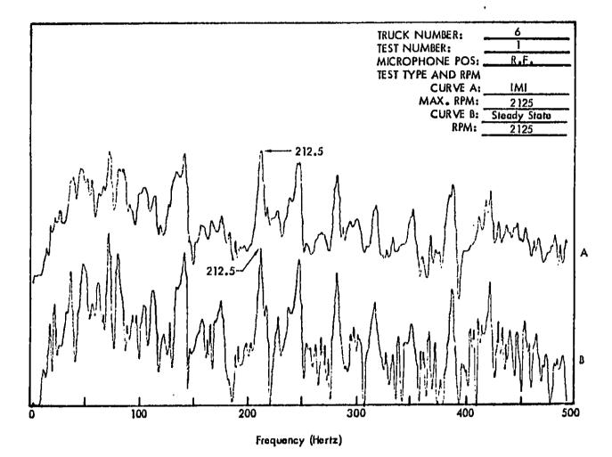
Figure C13. Truck Exterior Noise Spectra (Narrow Band Analysis 1–1/4 Hertz) Measured at 50 Feet. The Spectra Are Used For Determining Engine RPM.
