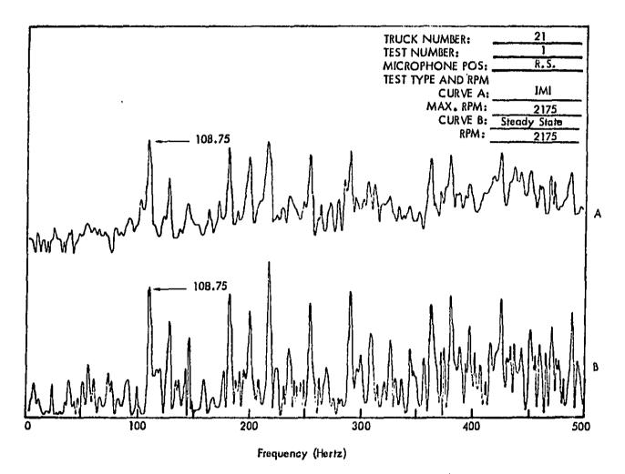
Figure C53. Truck Exterior Noise Spectra (Narrow Band Analysis 1-1/4 Hertz) Measured at 50 Feet. The Spectra Are Used For Determining Engine RPM.
