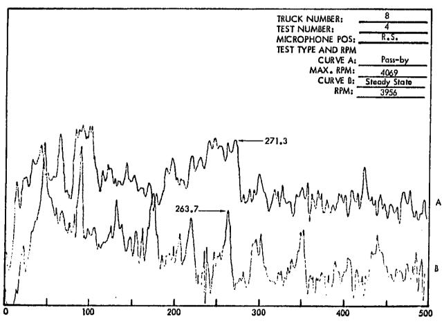
Figure C29. Truck Exterior Noise Spectra (Narrow Band Analysis 1-1/4 Hertz) Measured at 50 Feat. The Spectra Are Used for Determining Engine RPM.
