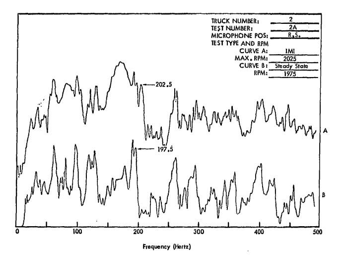
Figure C4. Truck Exterior Naise Spectra (Narrow Band Analysis 1–1/4 Hertz) Measured at 50 Feet. The Spectra Are Used For Determining Engine RPM.
