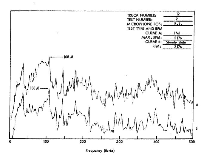
Figure C39. Truck Exterior Noise Spectra (Narrow Band Analysis 1–1/4 Hertz) Measured at 50 Feet. The Spectra Are Used For Determining Engine RPM.
