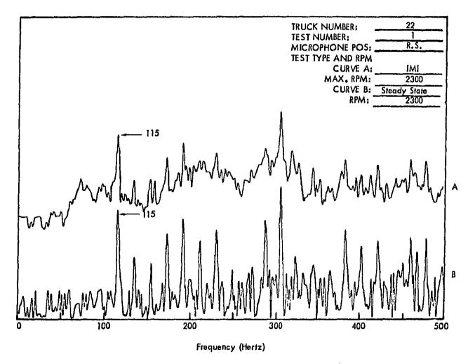
Figure C57 . Truck Exterior Noise Spectra (Narrow Band Analysis 1–1/4 Hertz) Measured at 50 Feet. The Spectra Are Used For Determining Engine RPM.
