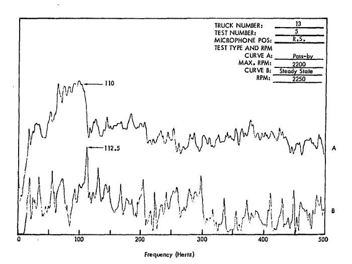
Figure C47. Truck Exterior Noise Spectra (Narrow Band Analysis 1–1/4 Hertz) Measured at 50 Feet. The Spectra Are Used For Determining Engine RPM.
