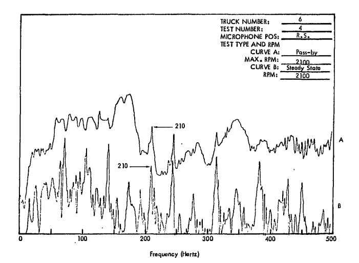
Figure C17. Truck Exterior Noise Spectra (Narrow Band Analysis 1-1/4 Hertz) Measured at 50 Feet. The Spectra Are Used For Determining Engine RPM.
