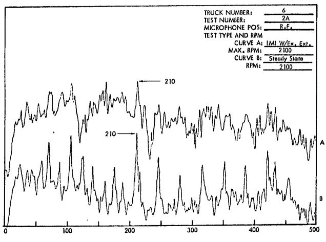
Figure C15. Truck Exterior Noise Spectra (Narrow Band Analysis 1-1/4 Hertz) Measured at 50 Feet. The Spectra Are Used For Determining Engine RPM.
