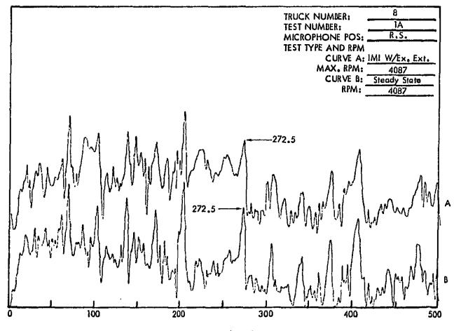
Figure C27 . Truck Exterior Noise Spectra (Narrow Band Analysis 1-1/4 Hertz) Measured at 50 Feet. The Spectra Are Used For Determining Engine RPM.
