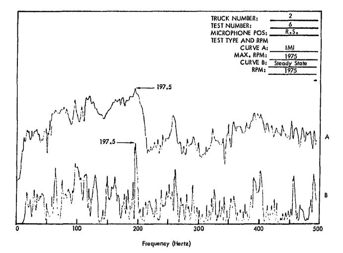
Figure C7 , Truck Exterior Noise Spectra (Narrow Band Analysis 1–1/4 Hertz) Measured at 50 Feet. The Spectra Are Used For Determining Engine RPM.
