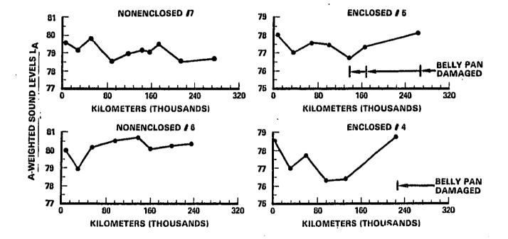
Figure 18. Vehicle Exterior Noise Levels versus Cumulative Kilometers Source: International Harvester (keference 6)
