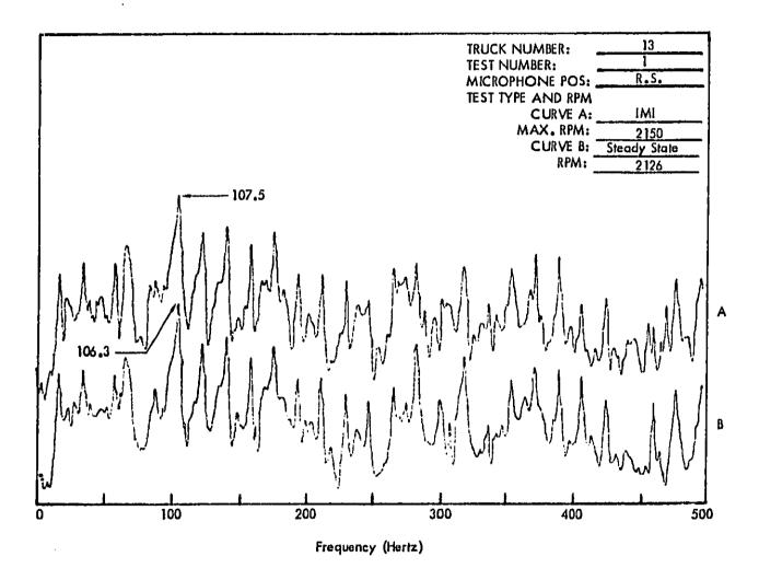
Figure C45 . Truck Exterior Noise Spectra (Narrow Band Analysis 1–1/4 Hertz) Measured at 50 Feet. The Spectra Are Used For Determining Engine RPM.
