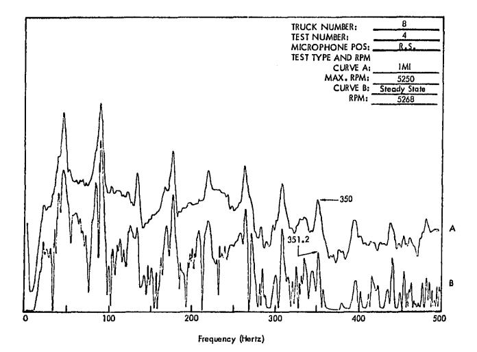
Figure C28. Truck Exterior Noise Spectra (Narrow Band Analysis 1–1/4 Hertz) Measured at 50 Feet. The Spectra Are Used For Determining Engine RPM.
