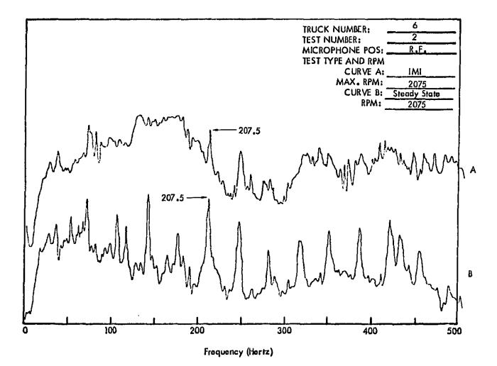
Figure C14. Truck Exterior Noise Spectra (Narrow Band Analysis 1-1/4 Hertz) Measured at 50 Feet. The Spectra Are Used For Determining Engine RPM.
