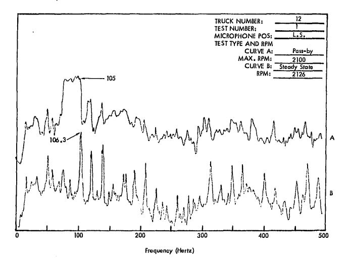
Figure C38 . Truck Exterior Noise Spectra (Narrow Band Analysis 1-1/4 Hertz) Measured at 50 Feet. The Spectra Are Used For Determining Engine RPM.
