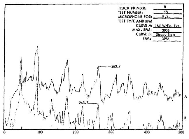
Figure C30. Truck Exterior Noise Spectra (Narrow Band Analysis 1-1/4 Hertz) Measured at 50 Feet. The Spectra Are Used for Determining Engine RPM.
