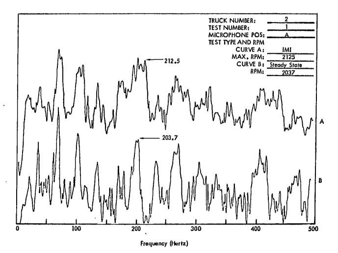
Figure C2 . Truck Exterior Noise Spectra (Narrow Band Analysis 1–1/4 Hertz) Measured at 50 Feet. The Spectra Are Used For Determining Engine RPM.
