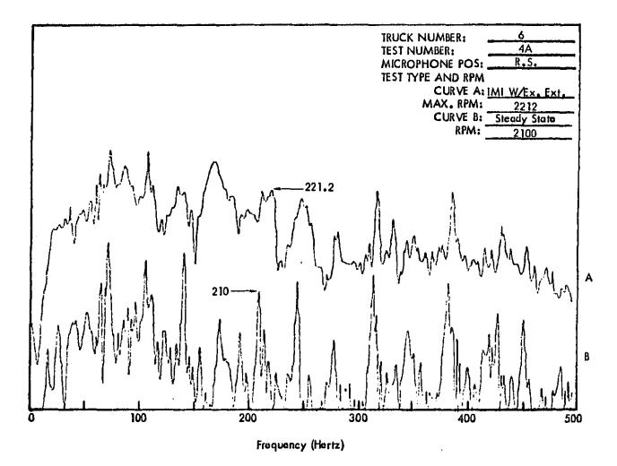
Figure C18. Truck Exterior Noise Spectra (Narrow Band Analysis 1-1/4 Hertz) Measured at 50 Feet. The Spectra Are Used For Determining Engine RPM.
