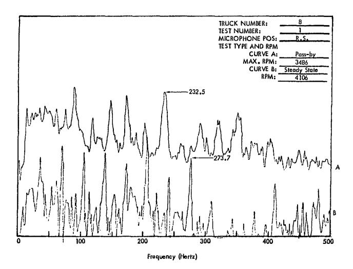
Figure C26 . Truck Exterior Noise Spectra (Narrow Band Analysis 1-1/4 Hertz) Measured at 50 Feet. The Spectra Are Used For Determining Engine RPM.
